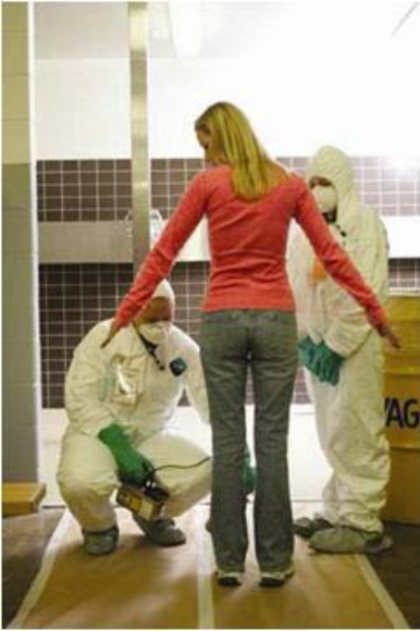
External Testing: Alpha/Beta/Gamma Emitters Pre-Decon
