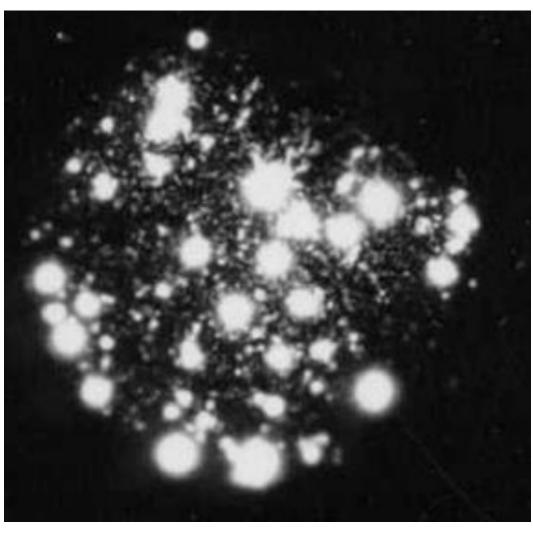
Sample grain size was 125 - 250 µm. The white spots are particles of plutonium while the entire dark area is due to soil particles without radionuclides.
