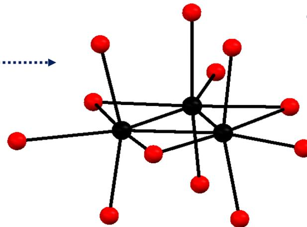
$\text{Tc}_3\text{Cl}_9$  cluster in  $\alpha$ - $\text{TcCl}_3$
