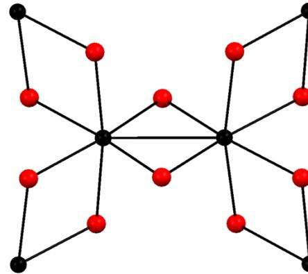
[Tc<sub>2</sub>Cl<sub>10</sub>] unit in  $\beta$ -TcCl<sub>3</sub>
