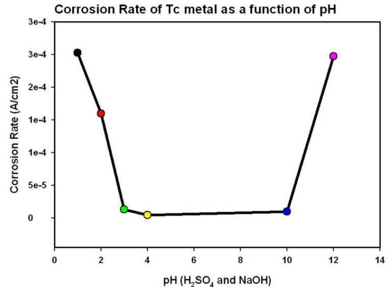
Corrosion rate as a function of pH mimics Tc(IV) solubility shape. Both may be used to estimate life-time of each phase.
