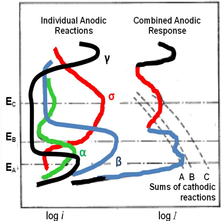
The Stern-Geary equation predicts that for  $E > E_{CORR}$  the anodic reaction predominates and for  $E < E_{CORR}$  the cathodic reaction predominates.
