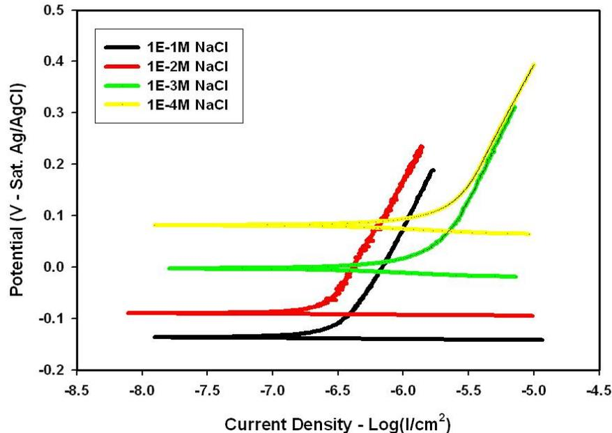
Alloy appears to be little effected by the presence of chloride on corrosion behavior, similar to Tc.
