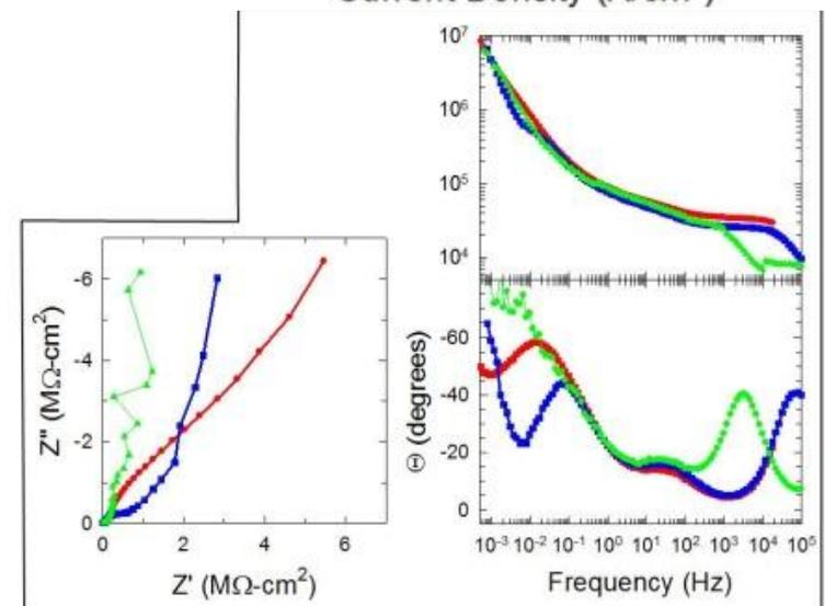
Increases in impedance observed as potential is ramped (EIS Red > Blue > Green lines)
