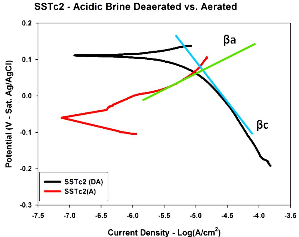
Effect of radical  $\text{O}_2^*$  formation should be minimized on the cathodic reaction, therefore predicting Tafel constant should be better estimated of corrosion rate.
