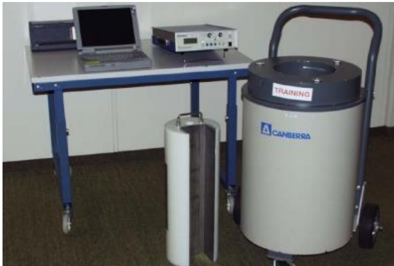
Active Well Coincidence Counter (AWCC)
