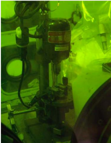
Figure 2.2. Miniature Drill Press for Coring CSNF Specimens Using a Hollow Stainless Steel Bit with Diamond Abrasive, Shown in the Hot Cell
