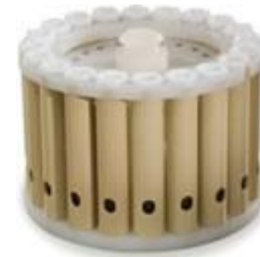
Q-20 Quartz Rotor Ultratrace analysis, high sample throughput Max. temp.: 250°C, Max. press.: 40 bar
