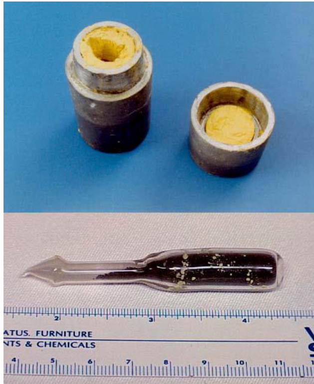
Lead pig and HEU oxide sample interdicted in Rousse, Bulgaria in 1999 (Kristo, 2011).
