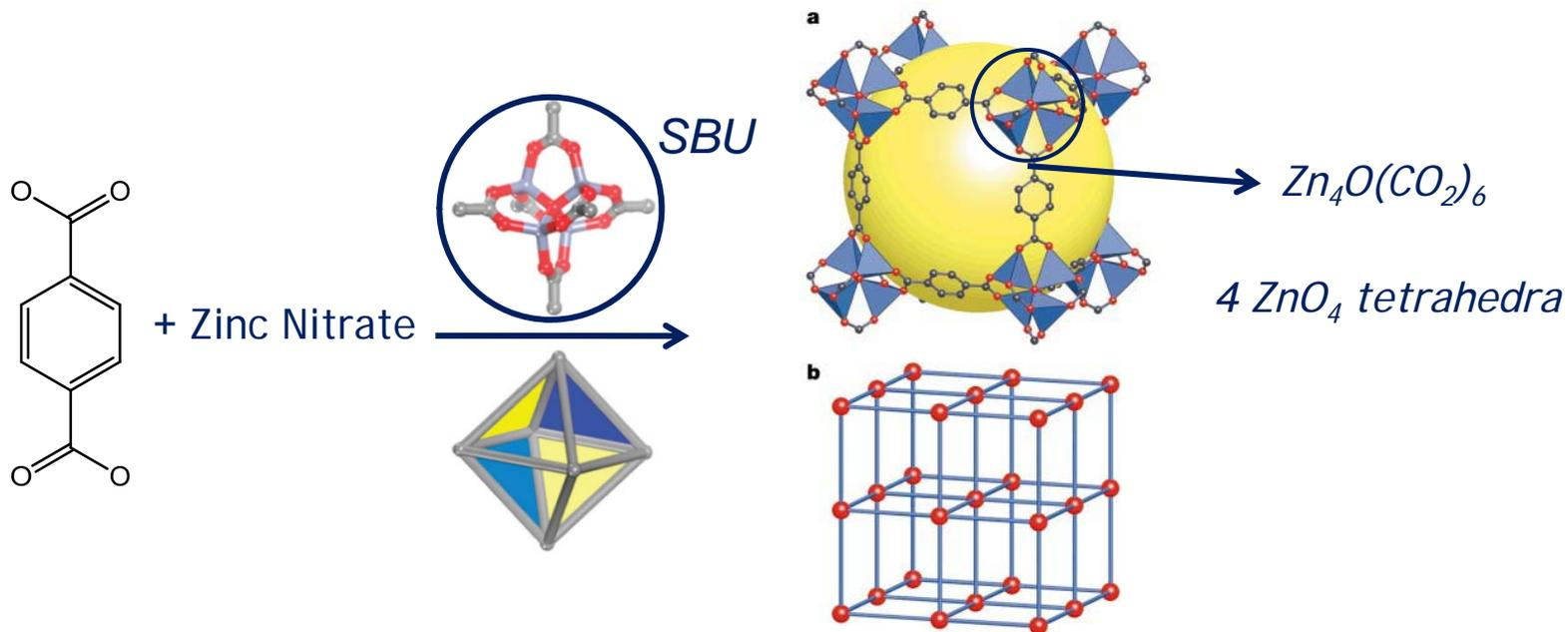
✓ The use of multiple metal ions in a cluster bridged by multiple coordinating ligands tends to enhance the robustness of the MOF
