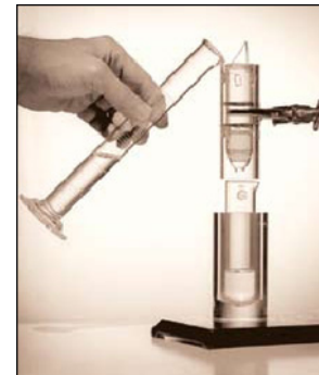
^{99}\text{Mo}/^{99\text{m}}\text{Tc} generator prepared by Tucker and Margaret Greene, 1958
